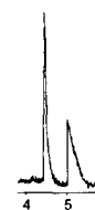
Fig. 8. Enantiomer separation of mianserine by CE using a 40 mM phosphate buffer (pH 3) containing 100 \mu M \gamma -CD-SBE. For other conditions, see Table 1 (cf. Section 3.3).
