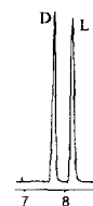
Fig. 9. Enantiomer separation of dansyl-leucine by CE using a 30 mM phosphate buffer containing 5 mM \gamma -CD-SBE and 10% (v/v) methanol. Capillary: polyacrylamide coated (Beckman Neutralcap), 37 cm \times 50 \mu m I.D., 30 cm injector to detector; voltage, -15 kV (reversed polarity).
